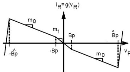
**Fig. 4.** Piece wise linear characteristic of the nonlinear resistor NR in Chua's circuit.
