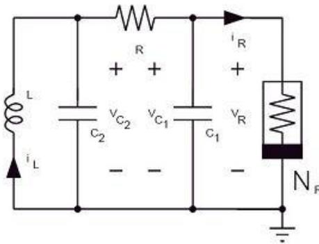
**Fig. 3.** Schematic of Chua's Circuit. NR is the active nonlinear resistor, called as the Chua diode.
