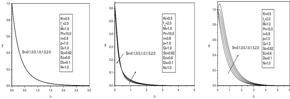
**Fig. 3.** Velocity, temperature and concentration profiles for different values of  $Sr$
