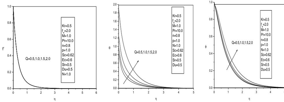
Fig. 5. Velocity, temperature and concentration profiles for different values of  $Q$
