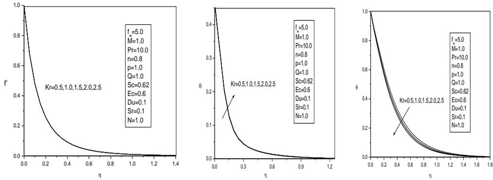
**Fig. 2.** Velocity, temperature and concentration profiles for different values of  $kr$
